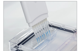
Multichannel pipettes can be used (31, 16 well combs)
